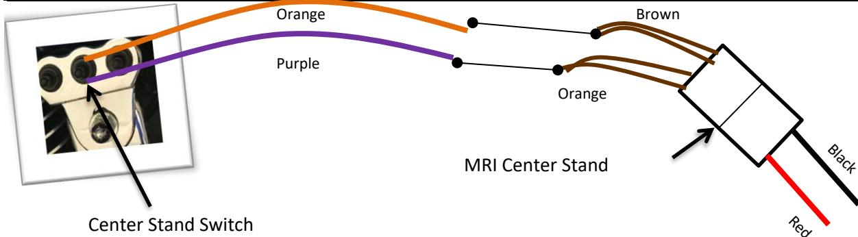
Tie both MRI Wires Together On Each Side Then Connect Them To My Purple & Orange Wires. Check Stand Operational Direction Before Soldering/Crimping Wires.
